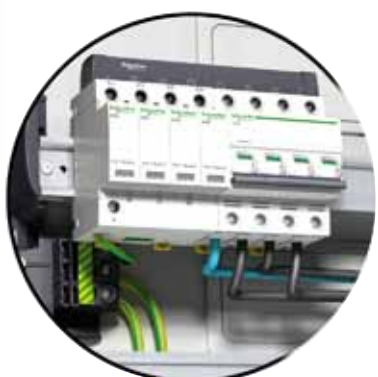
Surge arrester iPRD 4P + iC60N 4P for TNC-S or IT 230 V (L-L) with neutral, (Incoming through the bottom with comb busbar)
