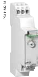
iRTB ■ Delays de-energizing of a load upon closing of an auxiliary contact (push button)
