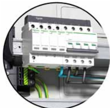
Surge arrester iPRD 3P+N + iC60N 3P+N for TT or TN-S (Incoming through the bottom with comb busbar)
