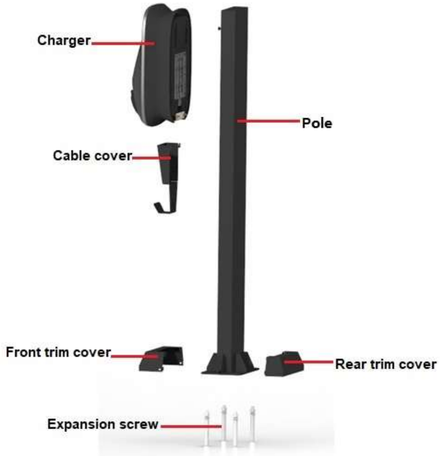
Figure A-16 Pole-mounted assembly drawing
